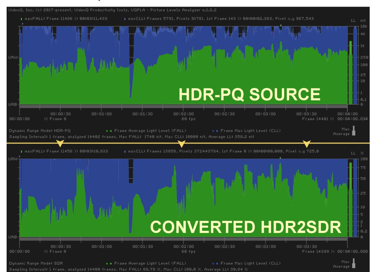
The *top half* of the image on the left is the **Light Levels Profile** of Netflix 'Nocturne' clip, UHD HRD-PQ 4 min long *input* fragment aka **HDR-PQ Source**.
