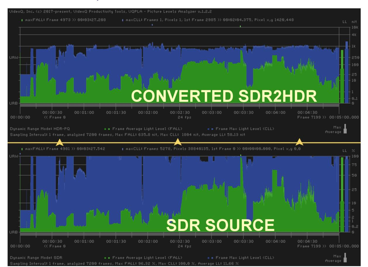
The *top half* of the image on the left is the **Light Levels Profile** of StEM2 'The Mission' clip, HD HRD-PQ 5 min long *output* fragment aka **Converted SDR2HDR**.
