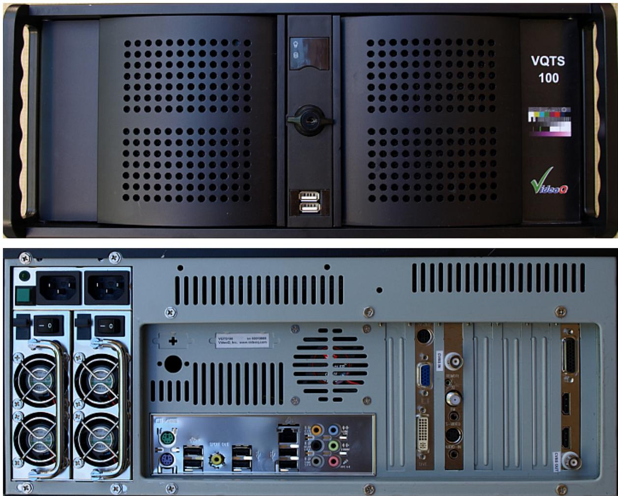
VQTS-100 is equipped with baseband analog NTSC/PAL CVBS video output and baseband analog NTSC/PAL CVBS video input.
