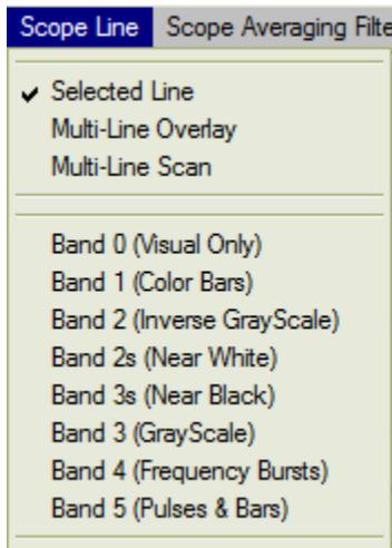
The easiest way to select displayed line is to choose the center of desirable Band by its name or number, for example - Band #1 = Color Bars.
