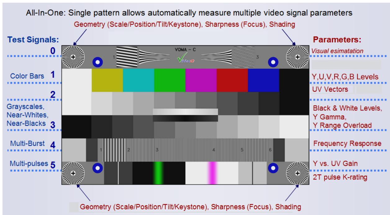
VQMA3 matrix consists of 6 horizontal bands (stripes) dedicated for automatic measurements of particular parameters. For convenience these bands are numbered "Band 0" to "Band 5" in VQMA3.EXE menus.
