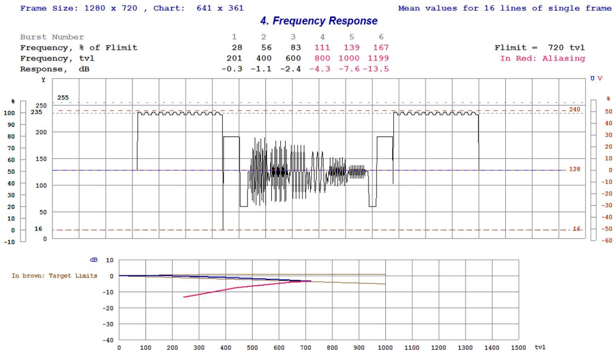
The list of burst frequencies tested by VQMA is rather short; 6 frequencies represent only few points on the frequency response plot. However, in typical test conditions frequency response plot shape is smooth. Thus, VQMA values, measured on few frequency bursts, adequately represent typical frequency response plot in total.
