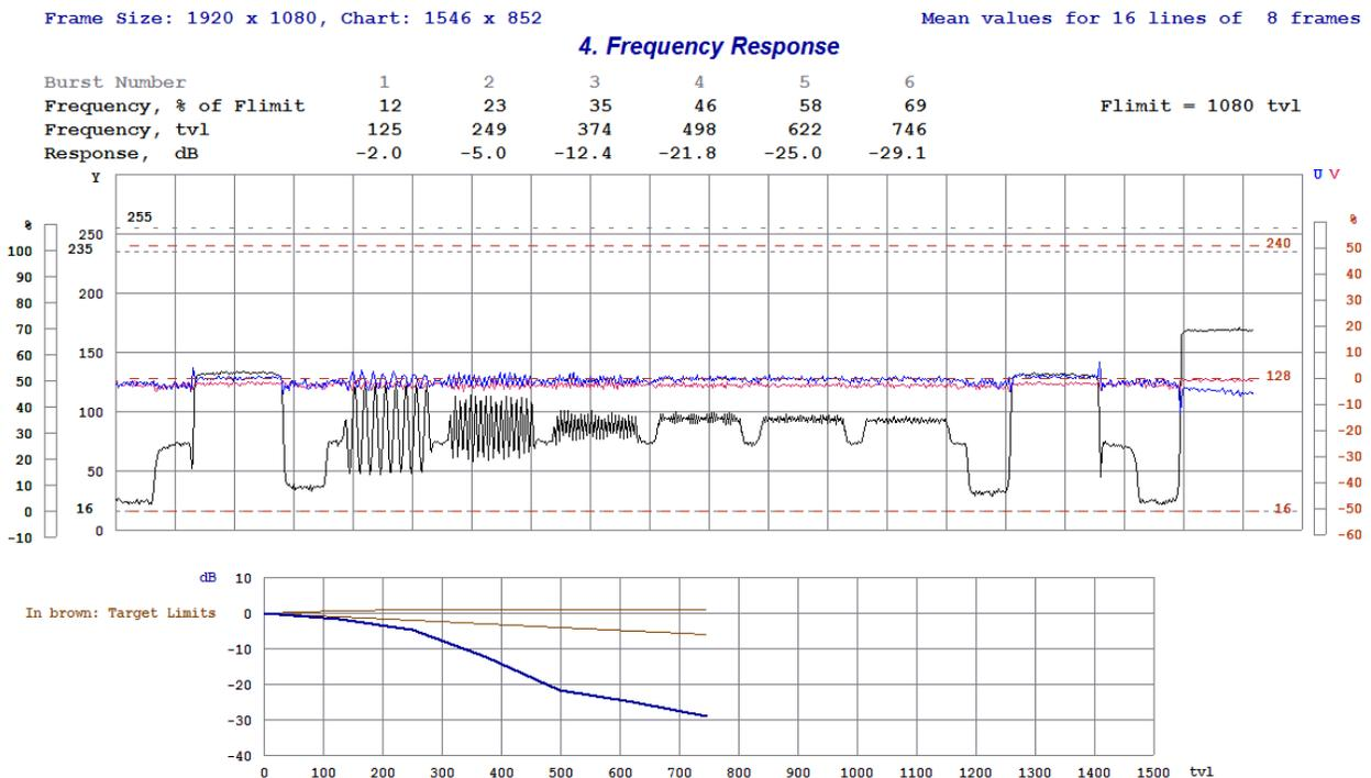
Waveform display on this page includes U (in red) and V (in blue) components useful for visual estimation of "debayering" ("de-mosaicing") algorithm artefacts. Strength of U and V variations appearing on monochrome textures provides an estimate of the debayering filter imperfection.
