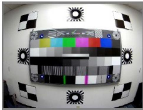
Even small **vibration** of the test chart will be *interpreted* by VQMA as increase of camera noise and drop-down of frequency response, so it is important to fix the chart firmly on something solid. Same applies to camera itself - any vibration during video data capture is highly undesirable. **Fluorescent light sources** are also undesirable. They produce **flickering light**, significantly biasing VQMA noise analysis results.
