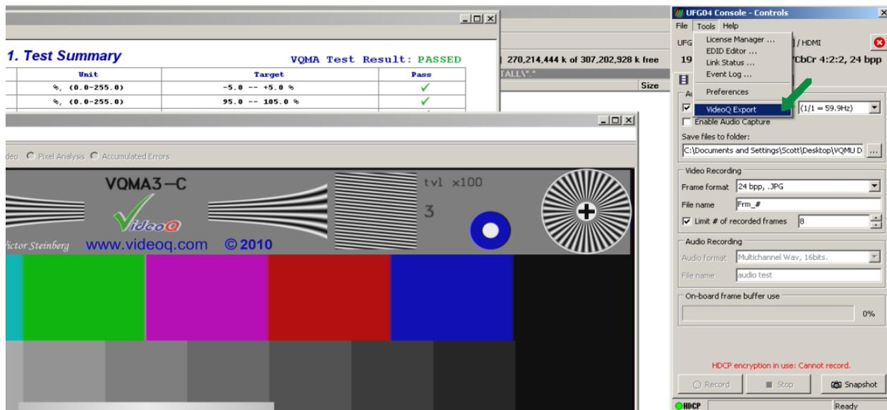
If HDCP restrictions are not present, it is possible to save YUV or BMP data files via Unigraf Console menus - instead or beside of launching VQMA analyzer.
