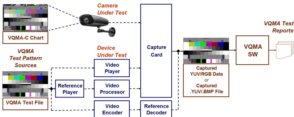
Captured test pattern video data should be stored on fast access media, e.g. HDD, in a file of suitable format, i.e. \*.YUV file or \*.BMP containing **single video frame or at least 8 consecutive video frames in uncompressed UYVY, YUV2 or RGB format with native 4:2:2 or 4:4:4 resolution** from minimum 640 x 480 to maximum 4096 x 3072.
