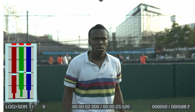
Non-adaptive conversion to SDR , such video is not acceptable. Massive clipping in the upper half – note overload indicators .
