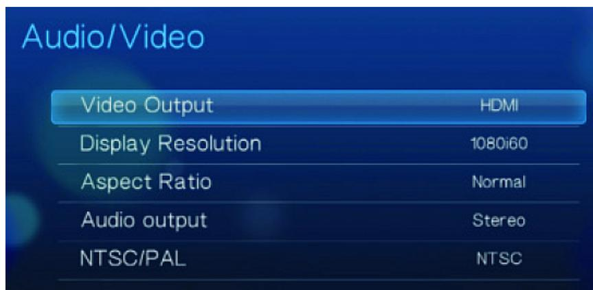
Selection of NTSC/PAL in "Settings/Audio-Video" sub-menu affects only the format of auxiliary analog CVBS output, it does not affect HDMI output.
