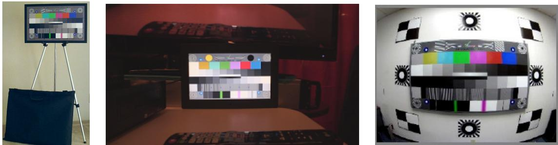
Even small **vibration** of the test chart will be *interpreted* by VQMA as increase of camera noise and drop-down of frequency response, so it is important to fix the chart firmly on something solid. Same applies to camera itself - any vibration during video data capture is highly undesirable. **Fluorescent light sources** are also undesirable. They produce **flickering light**, significantly biasing VQMA noise analysis results.
