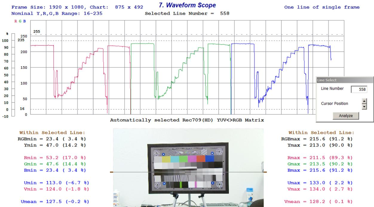
All YUV/RGB waveform diagrams are shown superimposed over the standard levels vs pixels grid.
