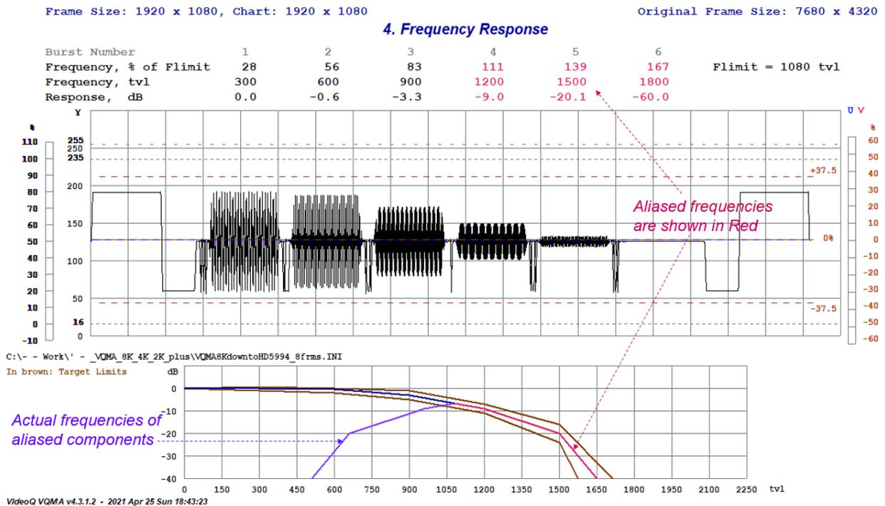
Beside main **Y** channel waveform the display on this page includes **U** (in red) and **V** (in blue) components useful for visual estimation of camera "debayering" ("de-mosaicing") algorithm artefacts. Strength of U and V variations appearing on monochrome textures provides an estimate of the debayering filter imperfection.
