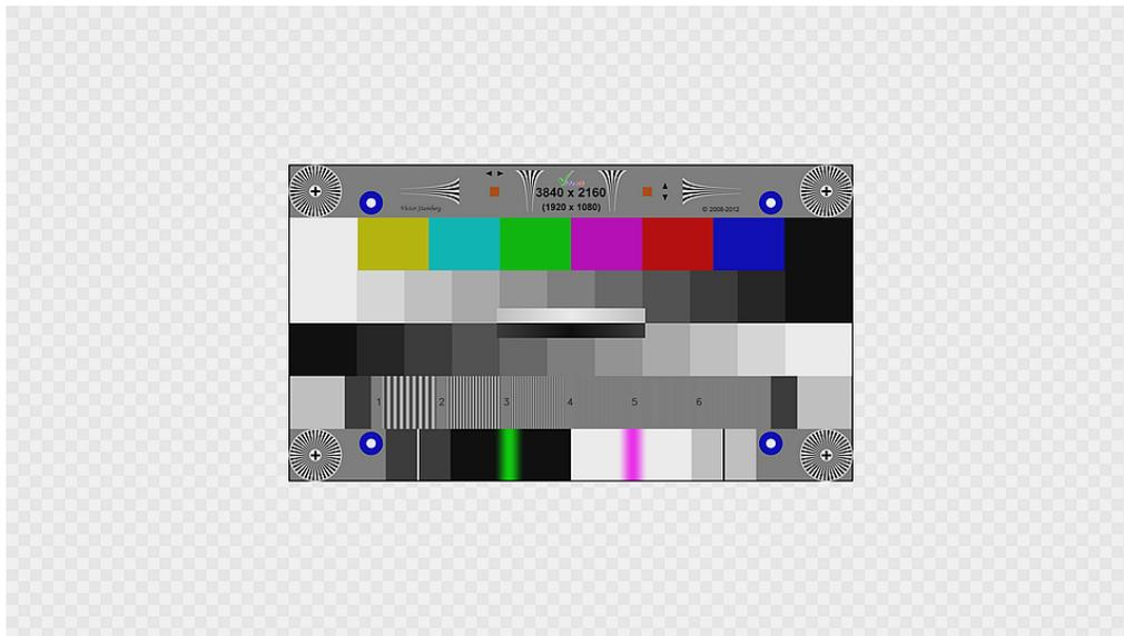
Such layout allows extension of measured frequency range. Spatial frequency of burst #6 is normally 600 tvl, but with reference to double height of UHD image it becomes 1200 tvl.
