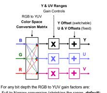
Full to Narrow conversion (shrinking the range, *default*): Y mapping gain = 219/255, UV mapping gain = 224/255 Narrow to Full conversion (expanding the range, *seldom used*): Y mapping gain = 255/219, UV mapping gain = 255/224
