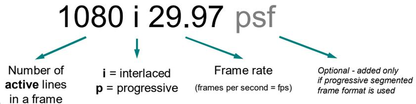
This naming convention can be also used for **full number of frame lines**, which includes the lines of vertical blanking intervals. For example, **625p50** and **1125i29.97** are absolutely correct names, if we talking about analog signals or digital SDI interfaces.
